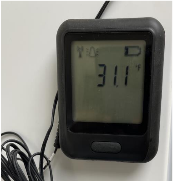
Out of range freezer temperature displayed on thermometer
