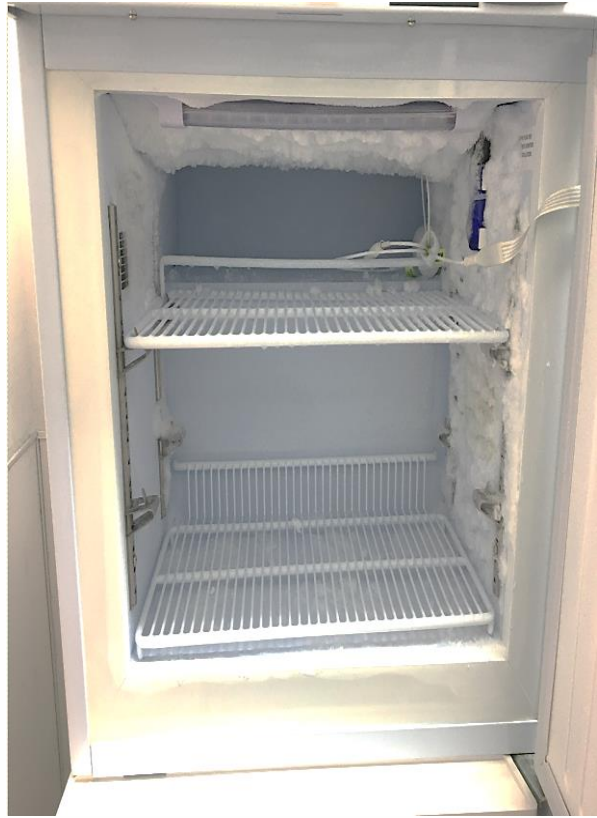
Ice build-up: Freezer needs to be defrosted
